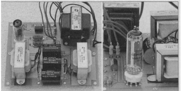
PHOTO 2: Assembled 300V B+ PSU.
