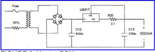
FIGURE 6: Heater PSU.
