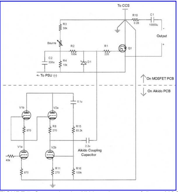
FIGURE 7: Connecting the Aikido to the source-follower MOSFET.
