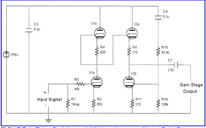
FIGURE 1: Tube Cad Journal Aikido gain stage. Note: Gain Stage Output.
